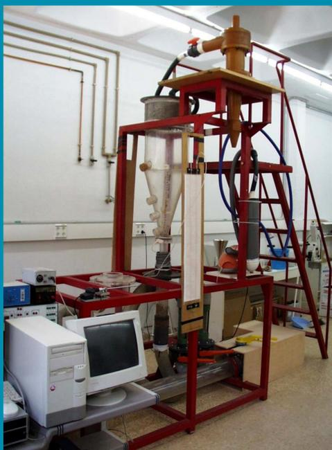
Experimental equipment with the conical spouted bed reactor
